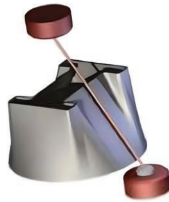
Figure.9 Example of part machining with Wire EDM
